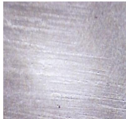
**Fig. VII.24** For 40 W, dissociation temperature is not reached on the target. No nano-structure form.
