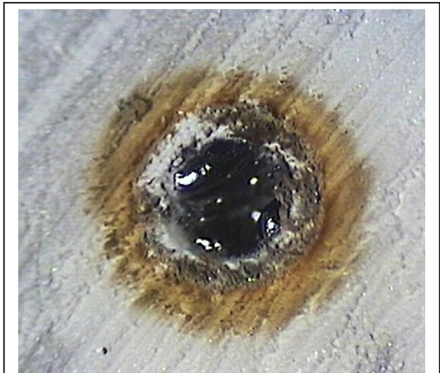
**Fig. VII.33** *The final impact, when target front surface has been polished by rough sand paper*
