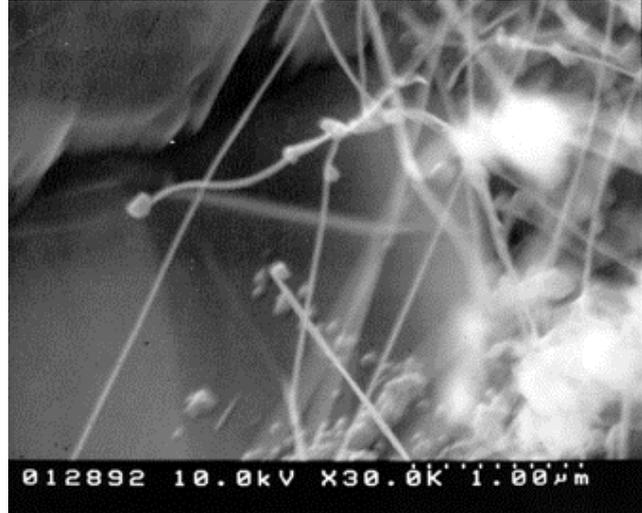
**Fig. IV.34 Seed-like ending at tube extremities (SEM)** Extremities are linked to the surface of a micro BN particle at surface of zone II. (From experiment at 50 mbar)
