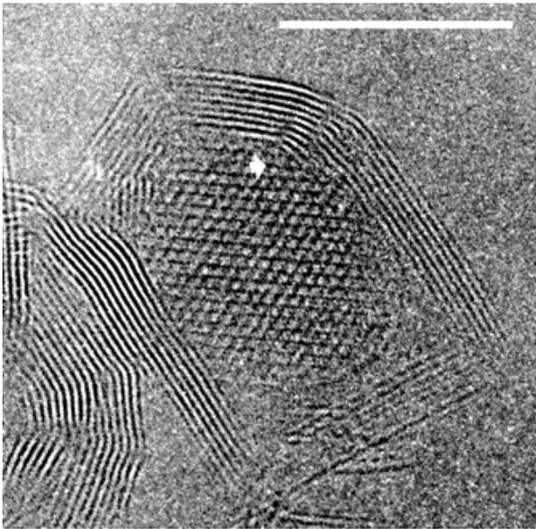
**Fig. IV.30** TEM imaging of a small BN nanopolyhedron containing a boron nano-crystal (in zone II) (direction 0001, hexagonal indexing). New layers of BN seem to be emerging from the boron core (arrow) in a process of combination with nitrogen from atmosphere. Several defects are observable in the shell. It merged on left side with another particle. Scale bar 10 nm. (Photo for 300 mb experiment)
